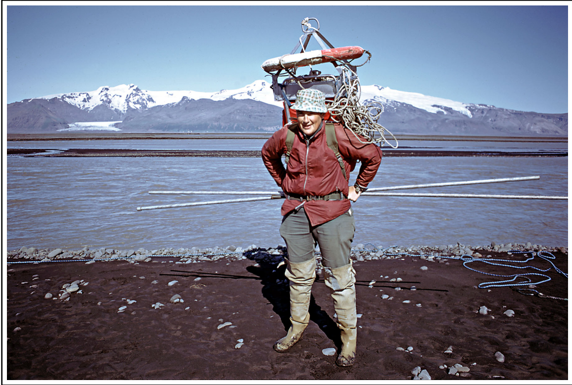
Caption: Jon on the Skeidararsandur (glacial outwash, fan delta) next to the Skeidarar River in summer of 1973. The gear he is packing was used to make current-meter measurements in the river. The pipes were buried in the outwash and used as anchors from which to tie ropes to in order to secure the rubber Avon water craft (not pictured). We made the current meter measurements from the water craft. Photo taken by A.C. Hine.
